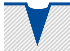
Honing structures filled with agglomerated solid lubricant
